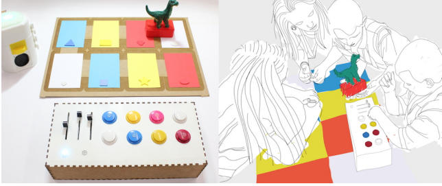
Figure 3: Left: the current story mapping prototype, with (clockwise) the scene module, the grid, the character module and the sampler. Right: children with mixed visual abilities interacting with the multisensory prototype.
